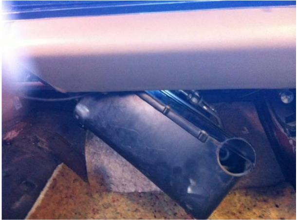
10) Once it comes away a few inches, remove the left and right discharge outlets to minimise their damage and space required to flip the heater box and get it out.
