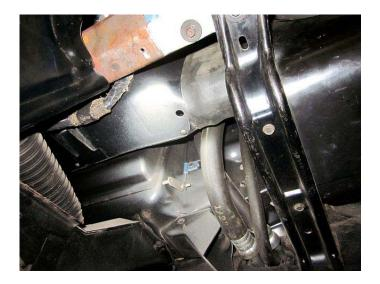
7) Remove the glove box liner and disconnect the RH duct going to the eyeball outlet or do it from underneath.
